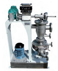
View of the Powder Hopper and FLOQUIP PSU 100 assembly
