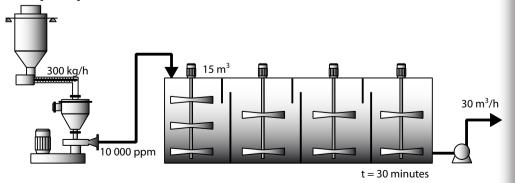
Typical Equipment Size Reduction between an equivalent installation with or without FLOQUIP PSU
