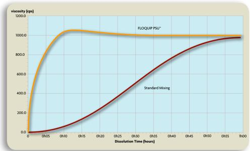
Graph 2: Viscosity as a function of the shear rate for polymer prepared by standard mixing and PSU dissolution
