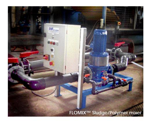
FLOMIX is most effective where the sludge is difficult to dewater, such as biological sludge on a belt filter and using a crosslinked flocculant (FLOPAM EM 4 BD/TBD). FLOMIX is also very useful on centrifuge applications where usually the dosages are always high (>20 kg/dry tonne).
