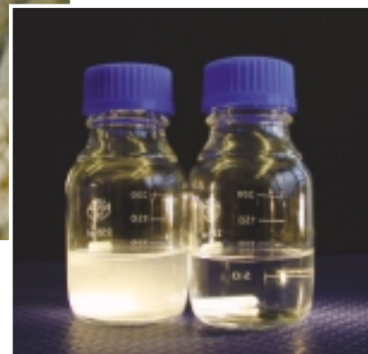
Struvite (Magnesium-Ammonium-Phosphate) in combination with sludge/polymer deposits.
