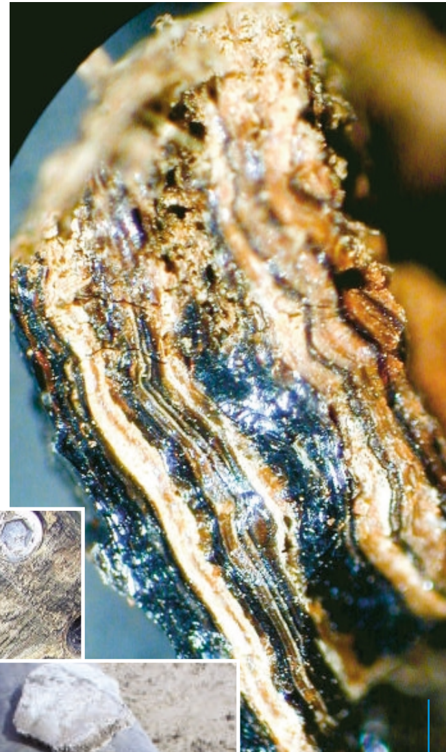
Microscope view of crystals layers (Struvite) [Mg(NH 4 )(PO 4 )·6H 2 O]
