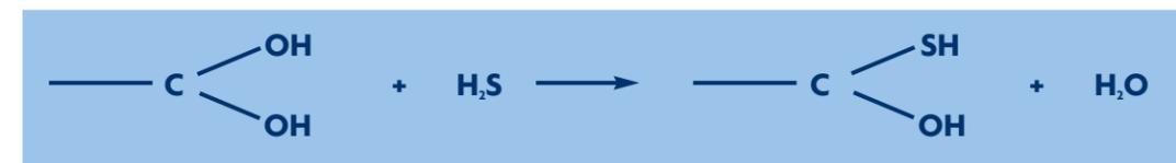
This range of products is particularly well adapted for high H<sub>2</sub>S levels, in a confined atmosphere (covered sewage plants, dehydrating room and sludge disposal). A maximum of 5 ppm H<sub>2</sub>S in air is allowed for an operator working 8 hours per day and only 10 ppm H<sub>2</sub>S is the maximum limit for someone staying 15 minutes in such an atmosphere. Where the H<sub>2</sub>S level is higher than this limit we recommend the use of **ODORFLO ACT** to react with hydrogen sulphide.
