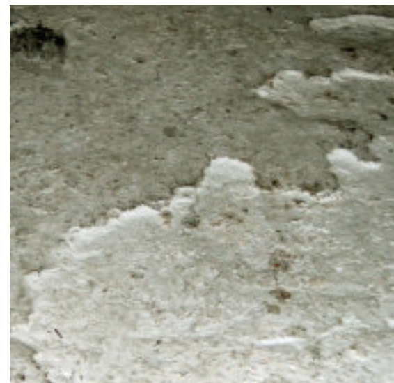
Hard polymer crust, thick and compact.
