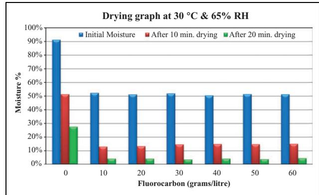
**Figure 5.** Drying graph of hydrophobic cotton.
