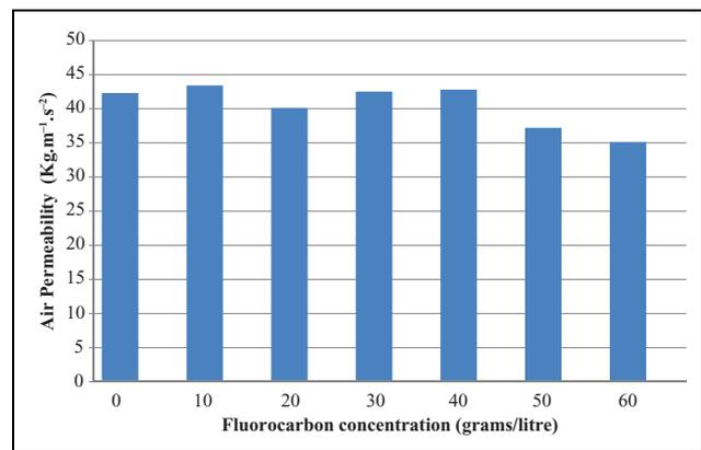
**Figure 6.** Air permeability of untreated and treated cotton with fluorocarbon at varying concentrations.
