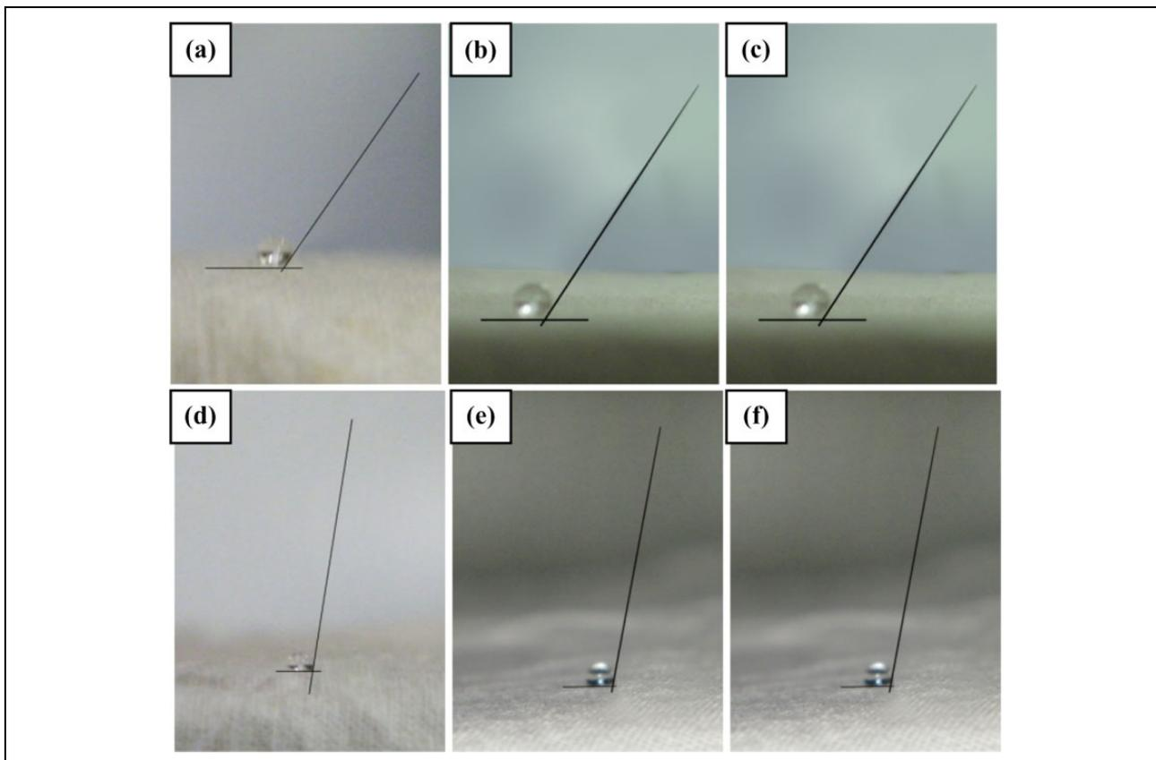
**Figure 2.** WCA of treated cotton with fluorocarbon before and after 20 washes. (a) 20 g/l unwashed WCA ( $123^\circ$ ); (b) 40 g/l unwashed WCA ( $123^\circ$ ); (c) 60 g/l unwashed WCA ( $127^\circ$ ); (d) 20 g/l 20 washes WCA ( $98^\circ$ ); (e) 40 g/l 20 washes WCA ( $101^\circ$ ); (f) 60 g/l 20 washes WCA ( $101^\circ$ ). WCA: water contact angle.
